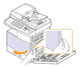
Pull the waste toner container out of the machine using its handle.
